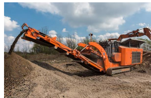
Recycling and valorization with a mobile crusher Publicworks deconstruction waste recycling platform
