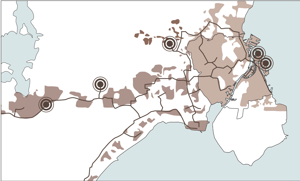
Copenhagen municipality and surroundings: waste incineration plants with their distribution networks for electricity and district heat.
