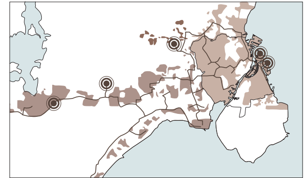
Copenhagen municipality and surroundings: waste incineration plants with their distribution networks for electricity and district heat.
